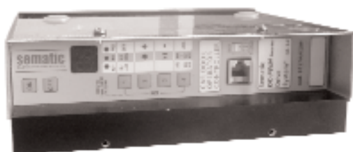
8 Complete a self-learning cycle of the Sematic Drive System® (Ref. 808-000-000 manual). This cycle must be carried out coupling the operator to a landing door. Out of the lock release zone of the landing doors, the device prevents the opening of the car doors.
